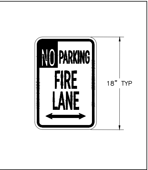
5 NO PARKING / FIRE LANE SIGN SCALE - NTS
