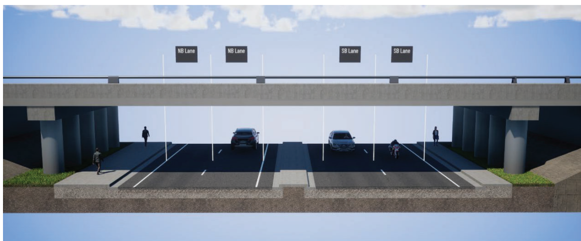
FIGURE 6: SUNSET DRIVE DDI TYPICAL SECTION UNDER I-94
