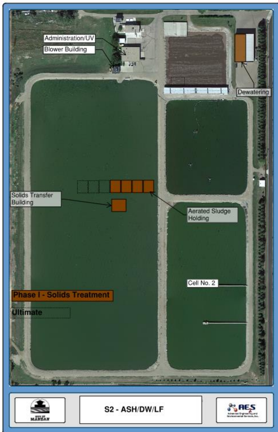
Figure 11 Solids Treatment Alternative 2 (S2)
